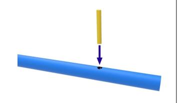
Carefully insert the heating elements through the holes in the insulation, taking care to locate the ends through the corresponding hole in the insulation at the other end of the furnace.
