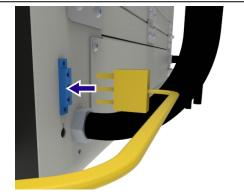
• Connect the female end of the lead to the end of the thermocouple.
