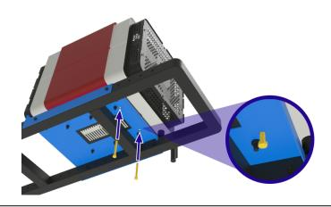
Using the appropriate lifting equipment, raise the furnace stand into a vertical orientation.
