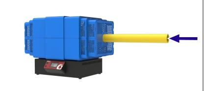
Adjust the positioning of the work tube until an equal length of tube protrudes from each side of the furnace.
