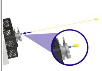
Connect the male end of the thermocouple lead to the socket at the rear of the furnace body.
