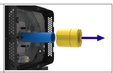
Slide the new insulation collar over the work tube until it is flush against the end of the insulation assembly.
