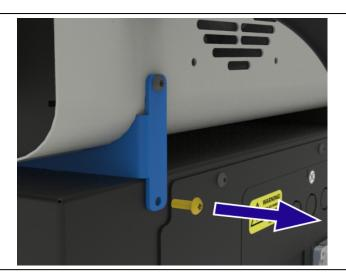
Slide the furnace body backwards to disengage the tabs on the spacer brackets from the slots on the top of the control box.
