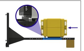
Insert the security screws through the back of the mounting bracket and into the base of the furnace to lock it securely in place.
