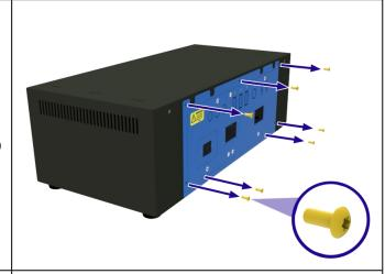
Carefully slide the panel out of the control box, and disconnect the earth connection, taking care not to disconnect or damage any wiring.
