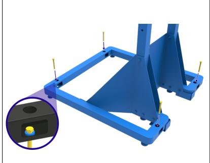
The vertical stands are supplied with a set of bungs that can be inserted into the bolt access holes in the base of the stand.
