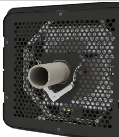
Refit the adjustment bar and securing nut, then gently tighten the support clamp assembly until it securely grips the work tube.
