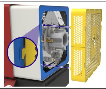
• Secure the end guard in place with a single screw
