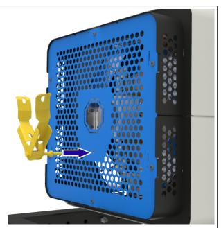
Insert the work tube into the furnace (refer to section 7.9), carefully sliding one end through the support clamp assembly so as not to damage the tube.
